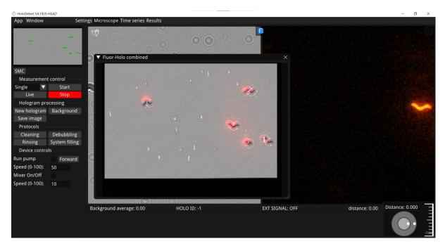
This offset has to be corrected using the built-in auto calibration routine. This requires the application of a sample that has objects with fluorescence (a sample containing alive algae is suitable). When the device is switched on or you want to calibrate the offset, please enable the auto calibration in the basic setting panel (see later).
